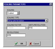
Activate scaling by setting the SCALING to Enabled.
