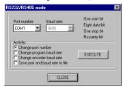
In the roll-down menu *Port number*, select the COM address to which the programming cable is connected.
