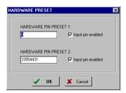
You can store any two position values as preset value 1 and preset value 2. To activate the two preset values, mark the corresponding control fields and close the window by clicking on *OK*.
